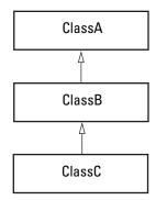
MATLAB always calls the most specific class constructor (ClassC in this case) first. This approach enables you to process input arguments and perform any necessary setup before calling the superclass constructors.
